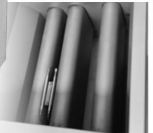
Fully peened tank ensures easy cleaning
